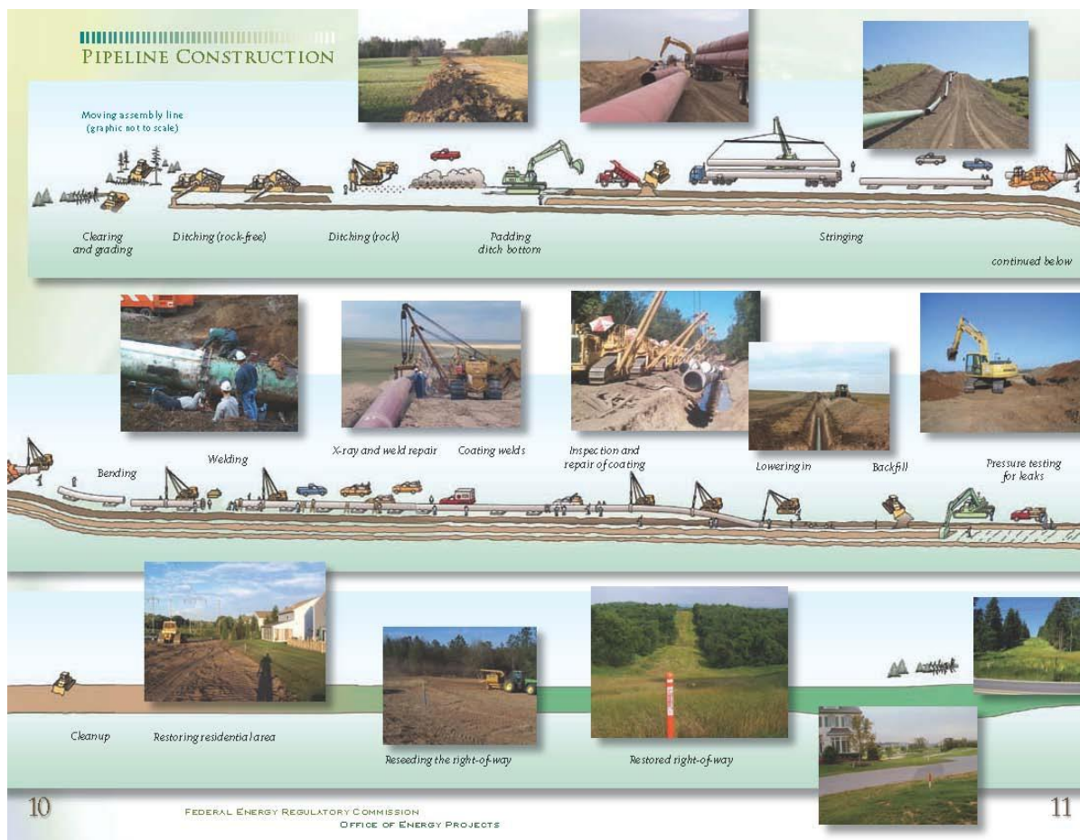
Figure 1.4-1. Typical Pipeline Construction Sequence
